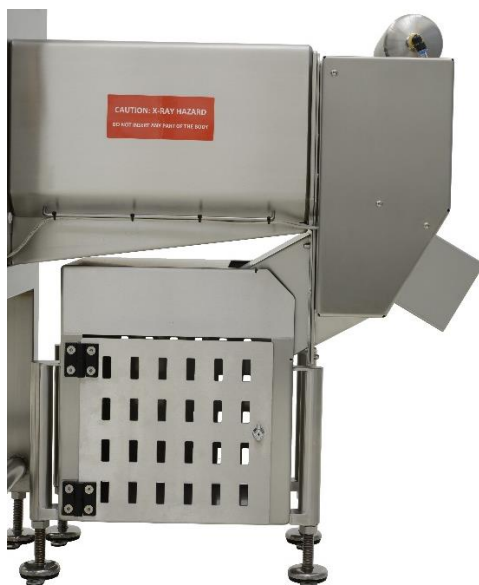
XRAY SHARK® reject system with rejection bin.
