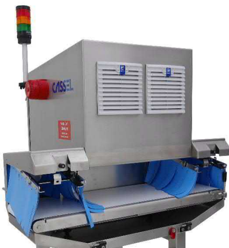
Removable double curtains for user protection and easy handling.
