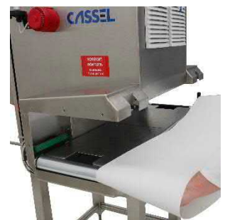
Remove conveyor belt.
