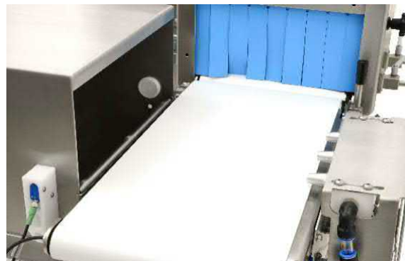
XRAY SHARK® XD28-L1 with air pressure reject system.
